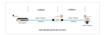
Diagram 2. UPoE+ Extender provides enough power to allow 300 metres (984 ft) of extension to a POE Plus wireless access point, using two UPoE+ Extender units located at 100 metre intervals.
