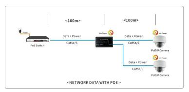
Diagram 2. PoE+ Extender provides enough power to allow 200 metres (656 ft) or 300 meters (984 ft) of extension to 3 POE IP Camera, using 2 PoE+ Extender units located at 100 metre intervals.
